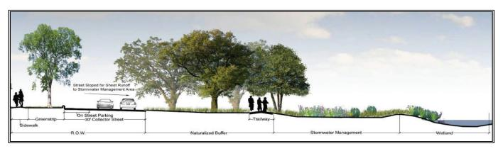
Figure 8. Stormwater Treatment Train within Conservation Development.
