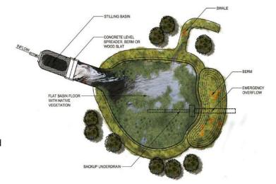
Figure 4. Naturalized dry bottom infiltration basin
