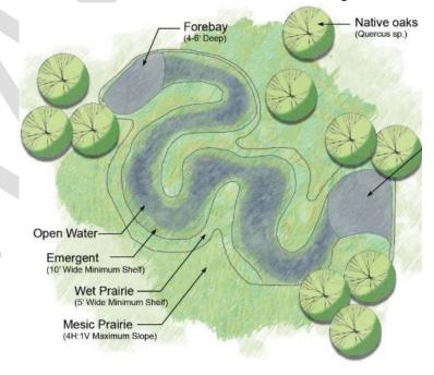
Figure 5. Naturalized wet bottom detention basin design.
