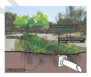
Dry vegetated swale rendering with engineered soils
